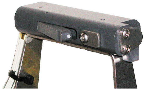
Figure 7 - Lock tab 180° from trigger
