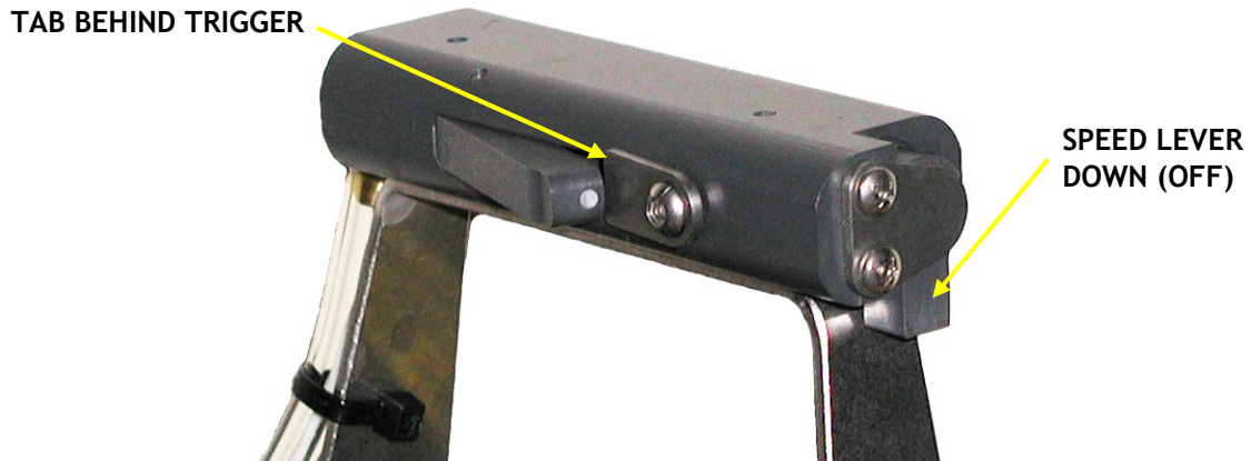
Figure 5 - Trigger locked off
